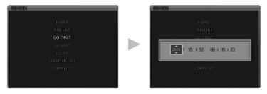
Users can enter a desired search date and time and press the PLAY button to playback. (The second setting can be input as 15 seconds/30 seconds/45 seconds.)
